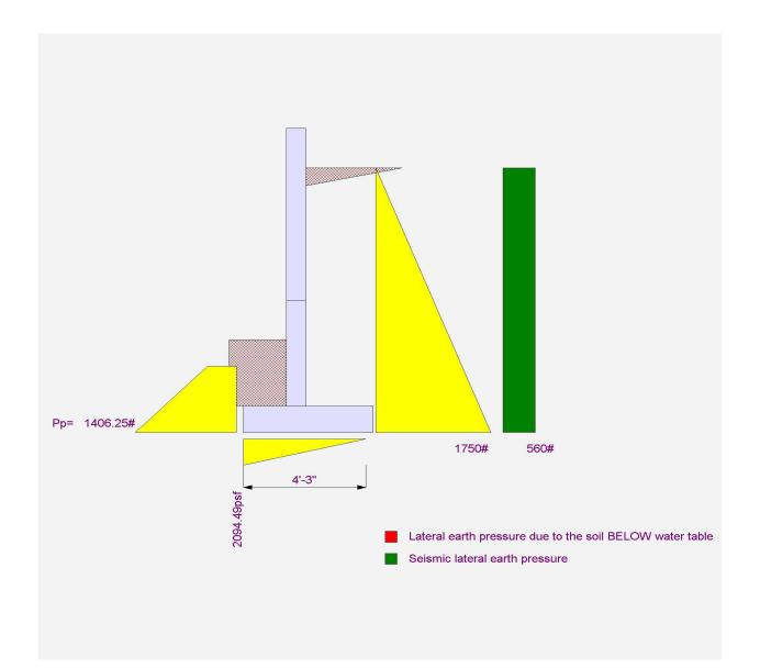
LIC# : KW-06017913, Build:20.23.04.05 MULHERN & KULP STRUCTURAL ENGINEERING INC **DESCRIPTION:** 9' CANT'D WALL @ SLAB
